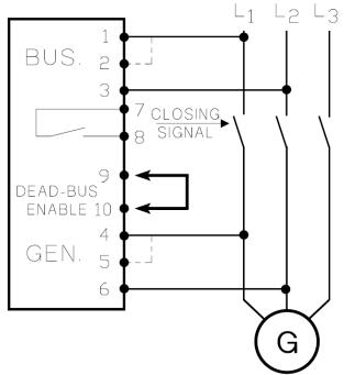
Before commissioning, make sure that the phase sequences of generator and busbar connections are correct.
